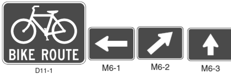
Figure 9: Bicycle Route Sign & Wayfinding Markers Illustration
