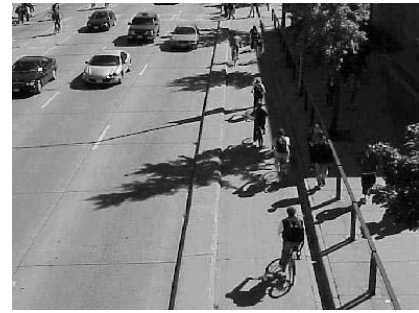
Figure 30. Separated Contra-flow Bicycle Lane. City of Madison, WI
